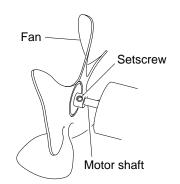
Figure 9 - Fan, Motor Shaft, and Setscrew Location
